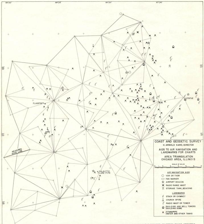
AN EXAMPLE OF THE NUMEROUS CULTURAL FEATURES WHICH ARE LOCATED BY THE COAST AND GEODETIC SURVEY IN THE PROCESS OF ESTABLISHING GEODETIC CONTROL THROUGH AN AREA. THESE PRECISE DETERMINATIONS OF POSITION FACILITATES THE ACCURATE CHARTING NECESSARY TO SAFETY IN AIR NAVIGATION; AND PROVIDES THE LOCAL SURVEYOR AND ENGINEER AMPLE BEARING FOR ORIENTATION OF HIS WORK.
